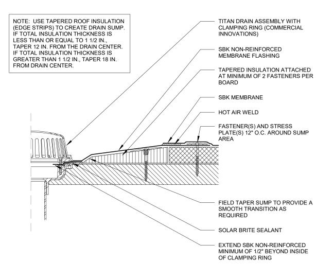
ROOF DRAIN FLASHING
